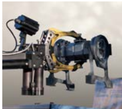
Claw rotates to easily grasp objects at difficult angles.
