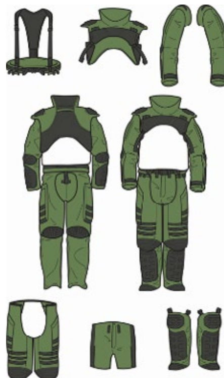
The TAC 6E is shown above with the lower leg protectors and the sleeves removed, to reduce weight, and in consideration of the threat.
